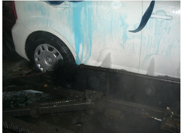
The creation of wheel brushes with varied filament lengths basically eliminates the need for labor or costly high-pressure sprayer systems to clean wheels.
